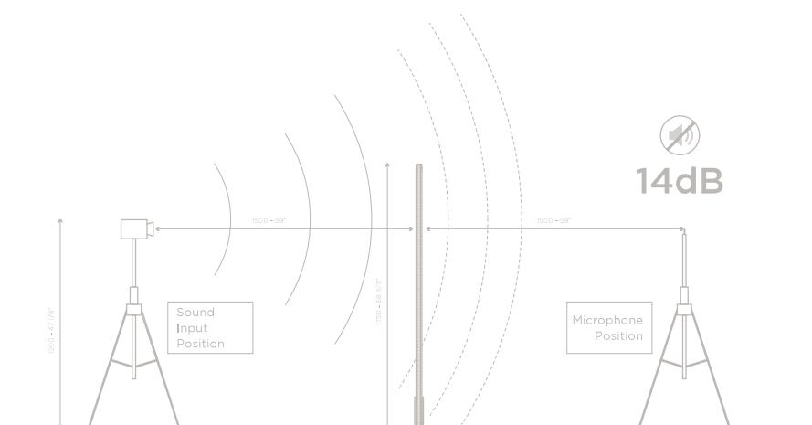
en\_Test effected on straight freestanding screen H=1750 mm, according to ISO 10053 regulation
